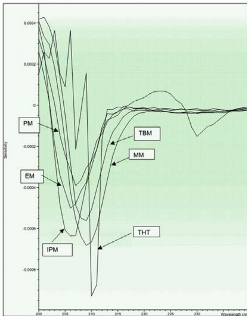
Figure 01: Derivative of absorbance spectra for different odorants in natural gas.
